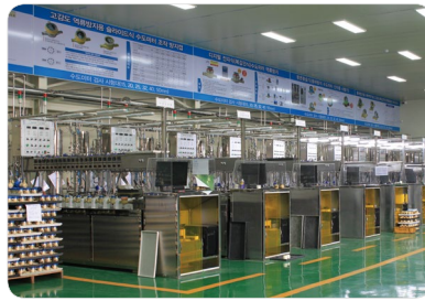
Full automatic water meter test 1,6 (multiple of 100 to 200) inspection table weighing & measuring function work (15 to 50 mm)
