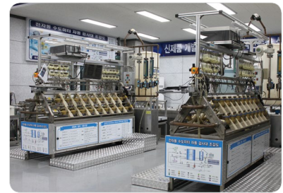
Full automatic water meter test 1,6 (multiple of 100 to 200) inspection table
